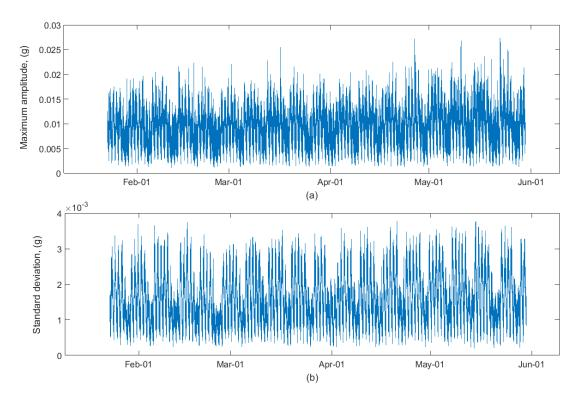
Figure 8. Time variation of statistics parameters for the selected vertical channel #20 on the Port Mann Bridge: recorded for three months from mid January to the end of May in 2018: (a) maximum amplitudes and (b) standard deviation.
