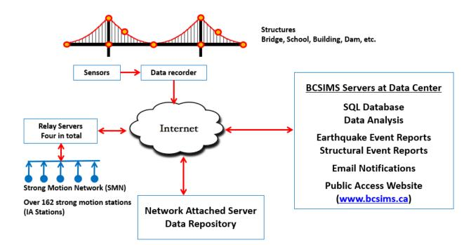
Figure 1. The components of the BCSIMS: servers, hardware and software, data acquisition system, data storage and processing tools, and network communications.
