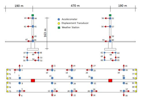
Figure 4. Instrumentation map for Port Mann Bridge (deck, towers and foundation only)
