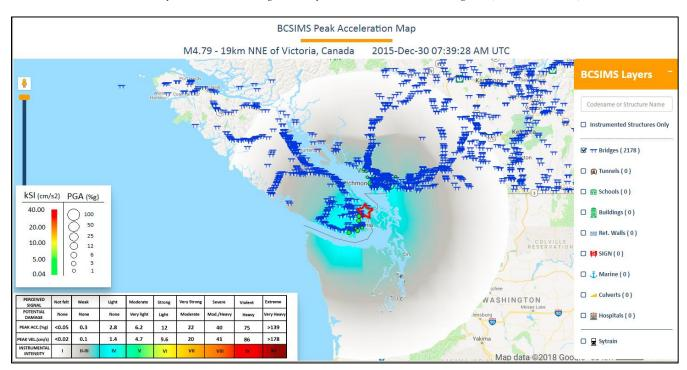
Figure 3. Calculated shake-map for the Mw4.79 earthquake that occurred near Sidney Island in BC, Canada. The location of the epicenter is indicated by a red star on the map, and the circles (50 in total) on the map show the locations of the triggered IA stations due that shaking (www.bcsims.ca).
