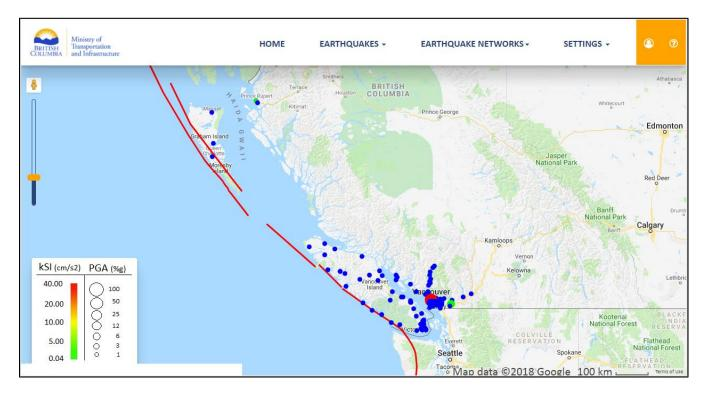
Figure 2. The IA stations (blue circles) are connected to the BCSIMS network in real-time. The size and color of the circles change in real-time based on the reported PGA and kSI values at that SM station. The size of the circle indicates the maximum measured PGA, and the color depicts the maximum calculated kSI value. This feature allows the user to immediately assess the shaking intensity in real-time across the region. (www.bcsims.ca)
